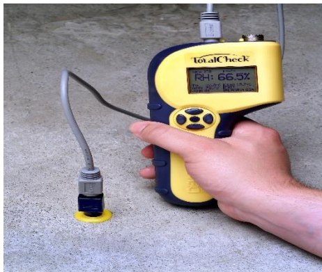
Moisture Floor Test
