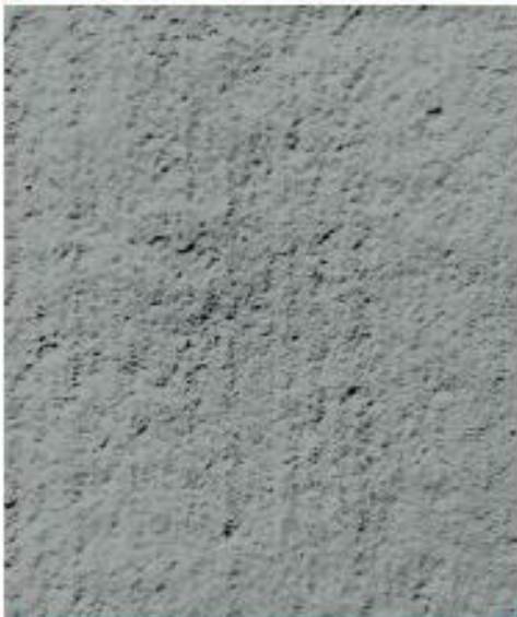
CSP 4 - Light Scarification
